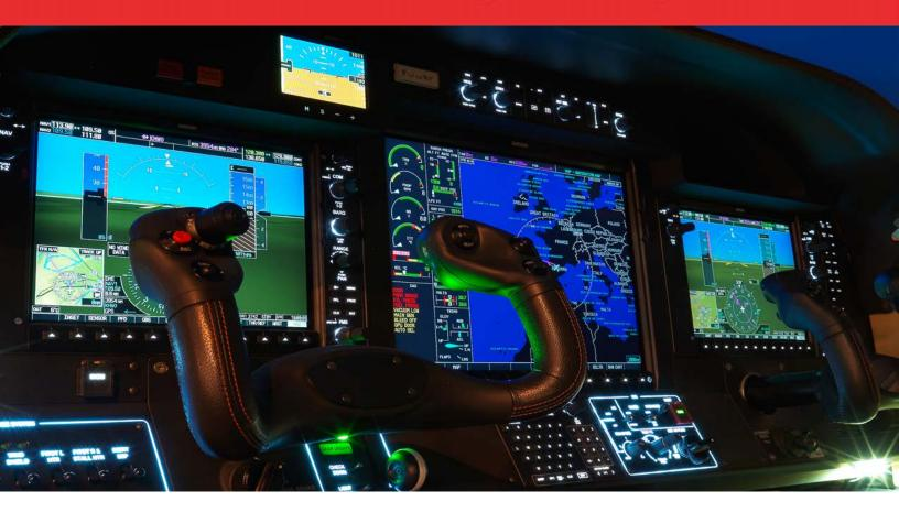
2 GMA 1347C Dual digital audio controller with integrated marker beacon receiver, intercom and public address capability on outer side for pilot and co-pilot side.
