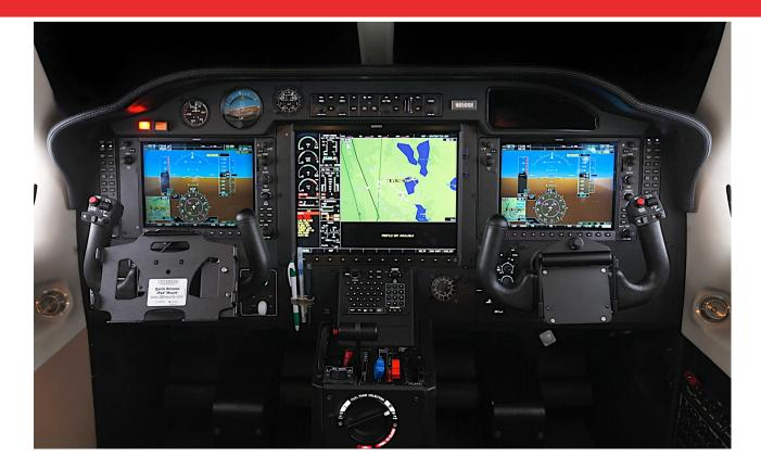
2 GMA 1347C Dual digital audio controller with integrated marker beacon receiver, intercom and public address capability on outer side for pilot and co-pilot side.
